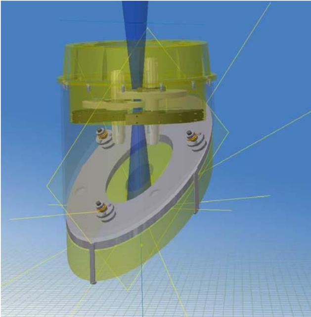
**Fig. 1** (online colour at: [www.an-journal.org](http://www.an-journal.org)) Constructional sketch showing the unit (green) in the shadow of the Nasmyth mirror (below). Blue: the beam with the focus F2 just at the position of the unit
