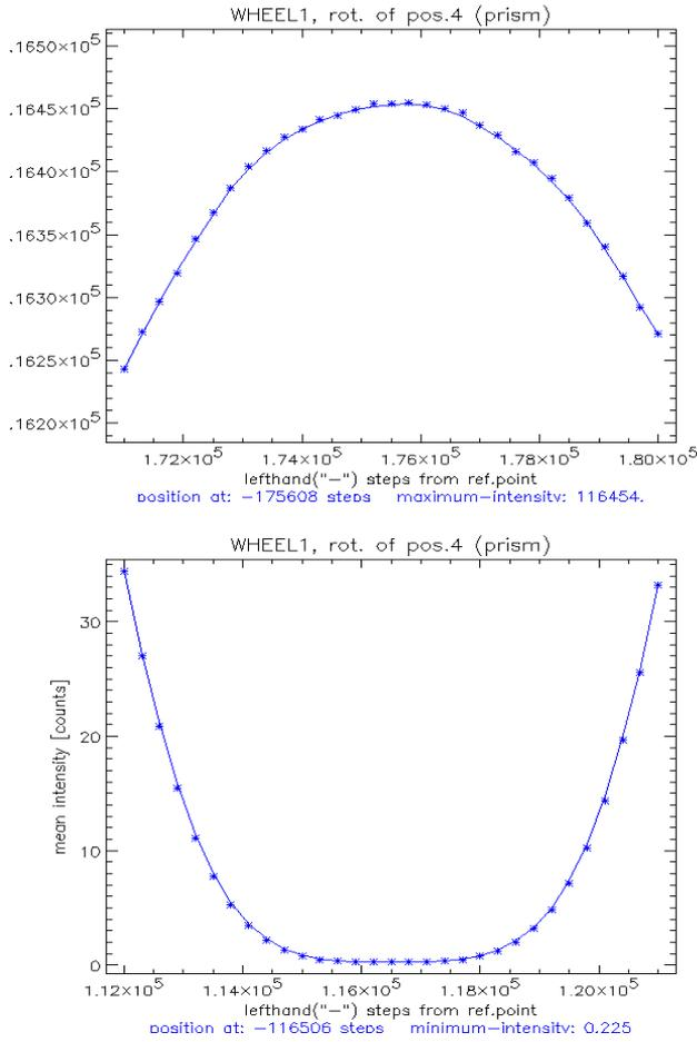
**Fig. 5** (online colour at: [www.an-journal.org](http://www.an-journal.org)) Intensities for rotating the prism in linear polarized light. *Top*: rotation around maximum transition; *bottom*: rotation around minimum transition.
