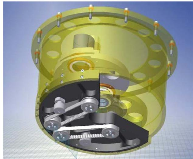
**Fig. 3** (online colour at: [www.an-journal.org](http://www.an-journal.org)) Constructional sketches of the unit. *Top*: front view showing the two wheels to insert and rotate different calibration optics into the beam. There are four micromotors (black cylinders) situated at the left hand to rotate the wheels and at the center of the wheels to rotate the mounts, respectively. *Bottom*: back view showing the gear belts and drives of the wheels
