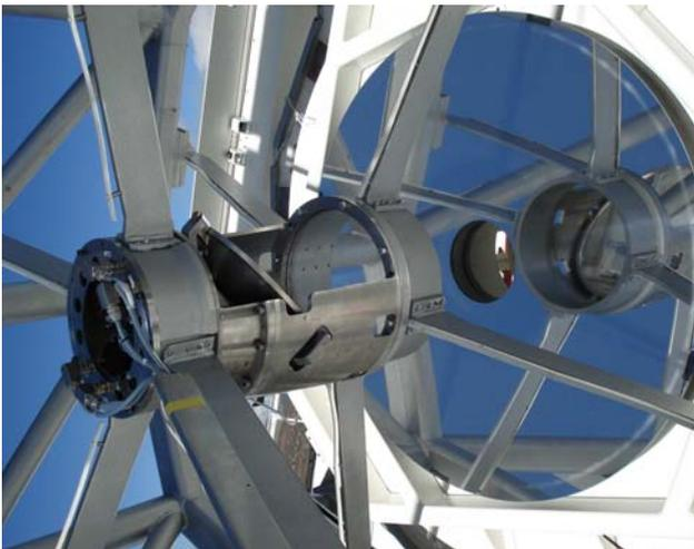
**Fig. 2** (online colour at: [www.an-journal.org](http://www.an-journal.org)) Position of the calibration unit next to the Nasmyth mirror M4 using the narrow beam close to the secondary focus F2, before the beam is reflected into the coudé axis.
