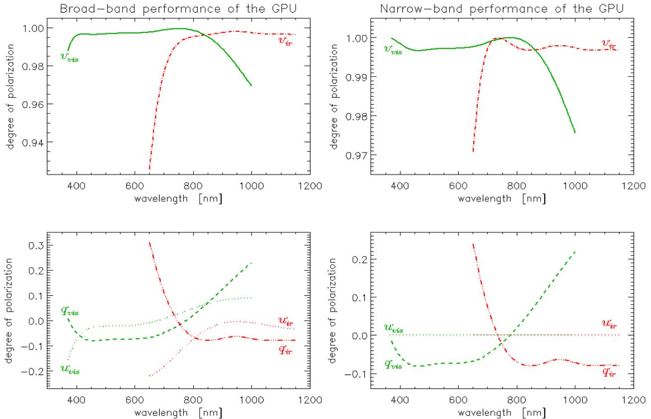
**Fig. 7** (online colour at: [www.an-journal.org](http://www.an-journal.org)) Wavelength dependence of the performance in generating circular polarized light. Green: using the retarder for the visible range, red: using the retarder for the infrared range.
