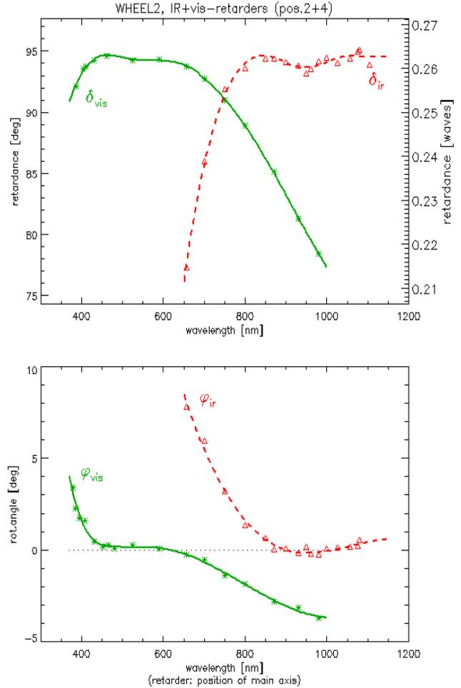
**Fig. 6** (online colour at: [www.an-journal.org](http://www.an-journal.org)) Wavelength dependence for parameters of the retarders (i) for the visible (green symbols represent the measurements and the solid lines are splines between them) and (ii) for the infrared (red symbols and dashed lines) spectral ranges. *Top*: retardance, *bottom*: orientation of the fast axis.
