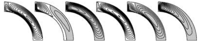
Figure 4. Contour plots of the R_B = 200 toroidal field at times 0.4, 0.42, ..., 0.5, with a contour interval of 0.01, and negative regions grey-shaded. The poloidal field is not shown, as it is essentially unchanged from \mathbf{B}_{p1} (which is only to be expected if b_3 never exceeds 0.15).
