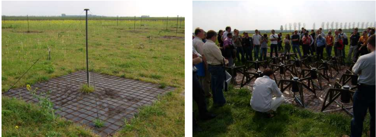
Figure 3: LOFAR low (left) and high (right) band antennae.
