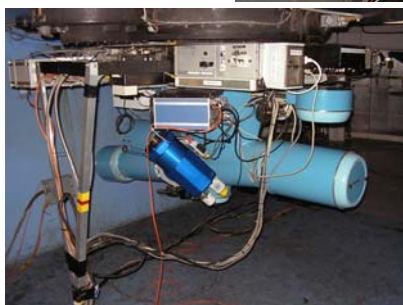
SOFIN is the high-resolution echelle spectrograph mounted at the Nordic Optical Telescope.
