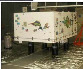
ESPaDOs is a bench-mounted high-resolution echelle spectrograph at the CFHT on Mauna Kea.
