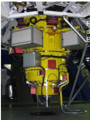
HARPS is the High Accuracy Radial velocity Planet Searcher at the ESO La Silla 3.6-m telescope.
