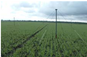
Fig. 1: LOFAR -antennas for radio wave lengths 4-10 meter (Figure: ASTRON Dwingeloo/ Netherlands)
