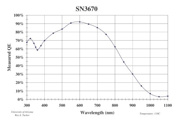
Figure 1. Measured QE at -118C
