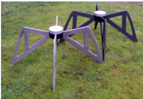
Fig. 2: LOFAR -antennas for radio wave lengths 1-3 meter. All 96 antennas of both types form one station. (Figure: ASTRON Dwingeloo/ Netherlands)
