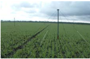
Fig. 1: LOFAR -antennas for radio wave lengths 4-10 meter (Figure: ASTRON Dwingeloo/ Netherlands)
