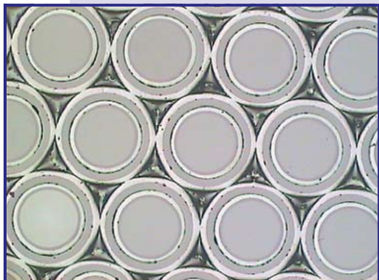
Fig. 4: Microscopic view of a section of the 2 nd fiber bundle for the Hobby-Eberly Telescope.
