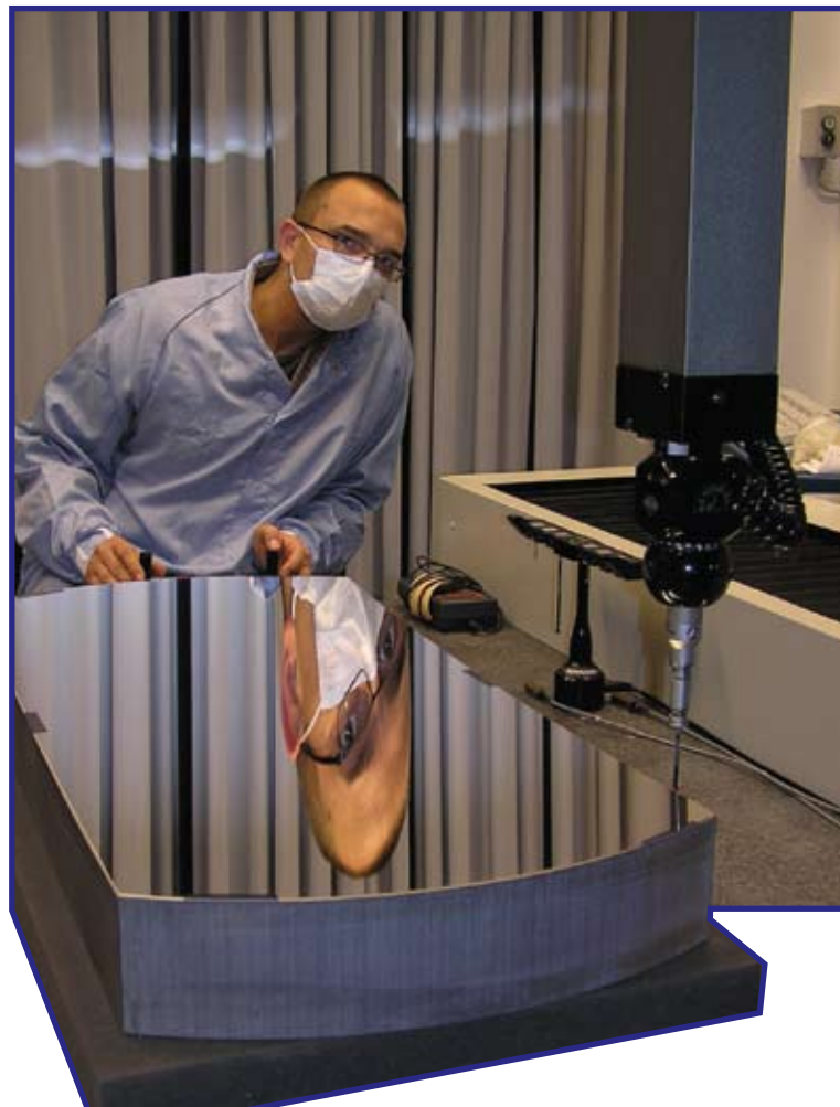
Fig. 2: Measuring the PEPSI collimator mirror in the optics lab.
