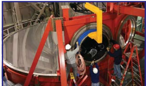
Fig. 8: The second AGW unit being mounted on the LBT in Oct. 2007.
