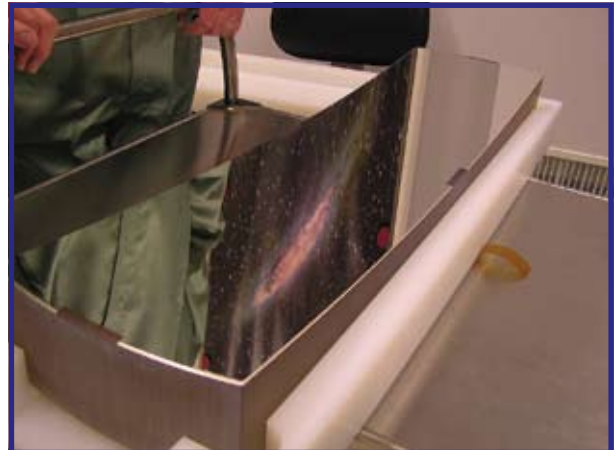
Fig. 10: Inspection of the red transfer collimator in the AIP clean room.
