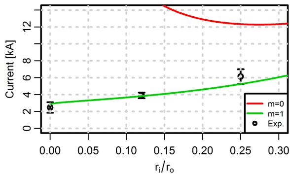
FIG. 5. Comparison of the determined critical currents with the numerical predictions for the  $m=1$  mode. The numerical prediction for the  $m=0$  (sausage) mode is indicated partly.
