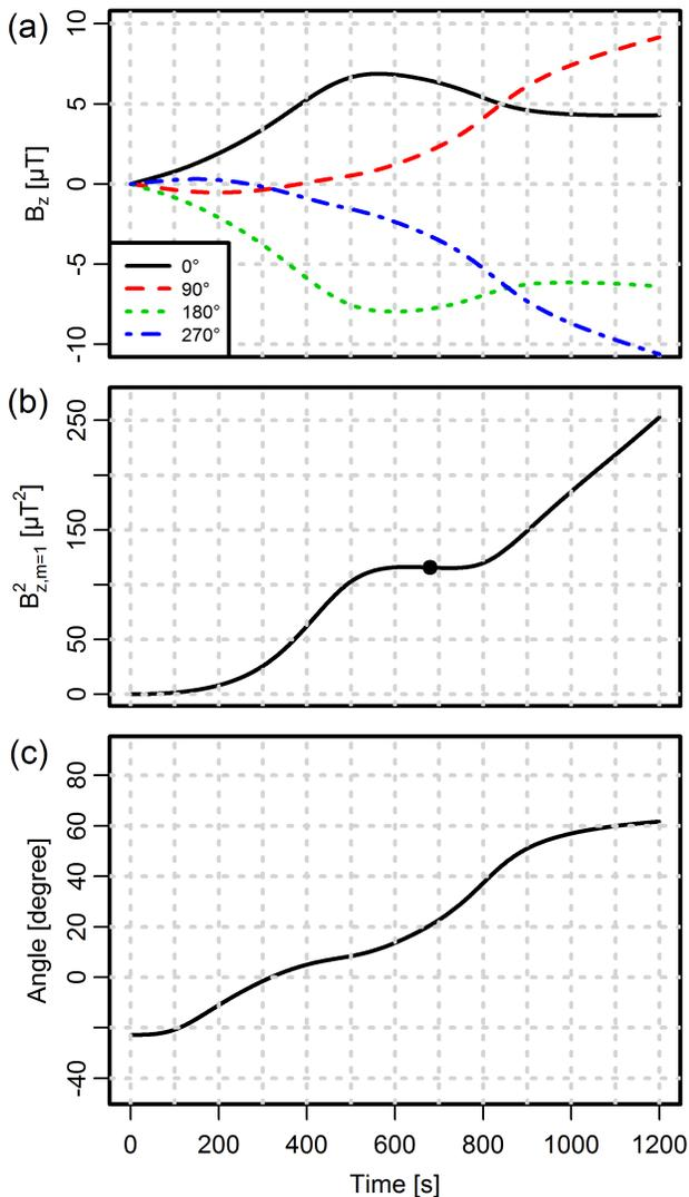
FIG. 3. Magnetic field data measured along the azimuth, for  $r_i=12.5$  mm and  $I=7$  kA. (a) Time dependence of  $B_z$  at the 4 fluxgate sensors. The  $m=1$  character is clearly visible. (b) Squared magnetic field amplitude of the  $m=1$  mode. (c) Angle of the  $m=1$  mode.
