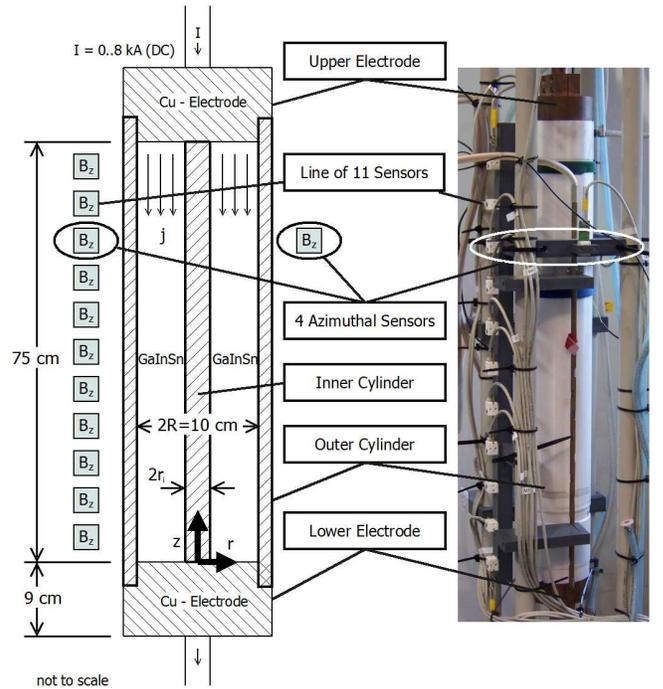
FIG. 1. Experimental set-up. Left: Scheme with liquid metal column and fluxgate sensors positioned along the vertical axis and the azimuth. Right: Photograph of the central part of the experiment.
