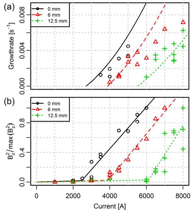
FIG. 4. (a) Measured growth rates and their numerical predictions for three different radii of the inner cylinder, in dependence on the current. (b) Measured squared magnetic field strength of the  $m=1$  mode, and their piecewise linear fits. The maximum squared fields for  $r_i=0$  mm, 6 mm, and 12.5 mm are  $61.0 \mu\text{T}^2$ ,  $543.3 \mu\text{T}^2$ , and  $1668.1 \mu\text{T}^2$ , respectively.
