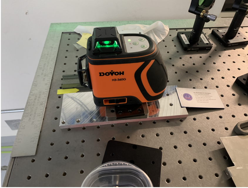
Figure 65: Image of the Dovoh H3-360G self-leveling green laser level used for table and beam height corrections.
