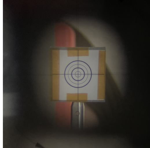
Figure 31: In the left image, the two targets placed at a distance of 8.55 cm are shown for both beam paths B3 and B4 . In the back behind the flipable targets is the theodolite. In this image, the theodolite focuses onto the second target from the left with the orange tape. The view of this target through the theodolite is seen in the right image. To be able to focus on this target, the flipable target needs to be flipped out of the beam path and the focus of the theodolite changed accordingly. Now the screws for the mirror alignment for mirror M2 can be corrected until the target is aligned to the cross-hair of the theodolite. For a perfectly aligned stage, the beam position should not shift when the stage moves.
