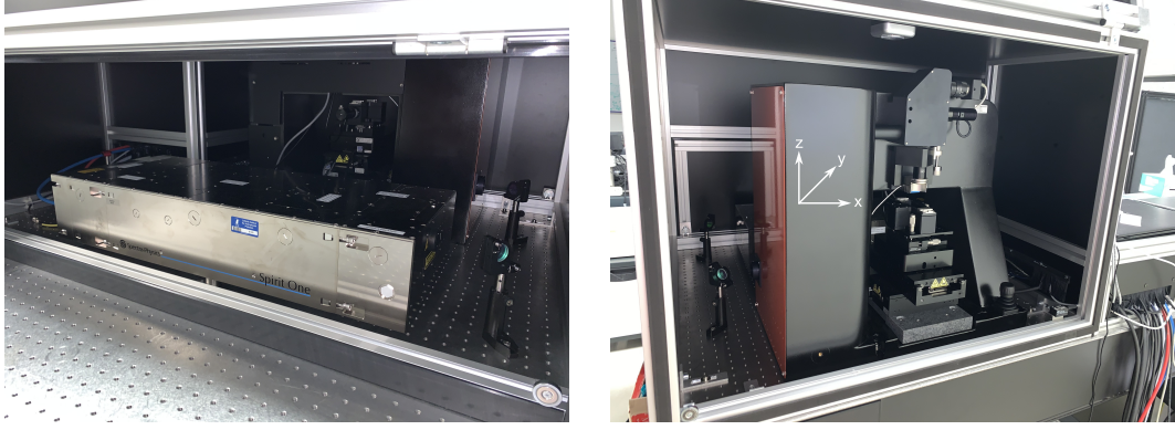
Figure 53: The ULI system at AIP is the commercial system FemtoFBG by MKS consisting of a femtosecond laser (Spirit One SPOne-8-SHG) (left), and an optics system as well as translational stages for the x- and y-axis (Newport, XMS100) and the z-axis (Newport, VP-5ZA) for automated waveguide writing. The ULI system is additionally equipped with a z-axis piezo stage (Piezosystem Jena, MIPOS 500). The femtosecond laser light is redirected to a vertical optics system hidden by the orange plate in the right image on the left side. The pulsed laser light is focused by a microscope objective, which can be mounted above the translational stages visible in the right image. Note that in the right image no microscope objective is currently inserted.
